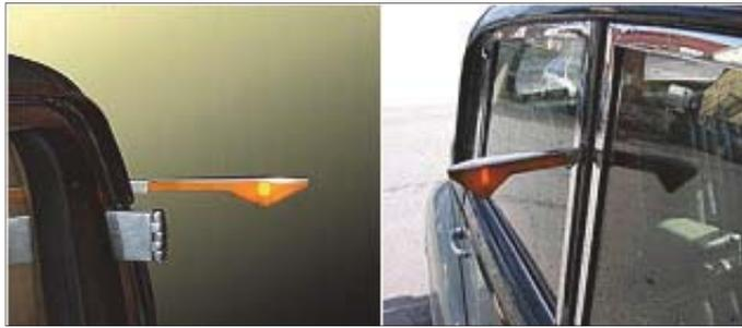
**Figure 1.** Trafficator in the "on" position
