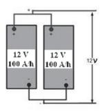
Fig. 1. Parallel connection of batteries (capacity 200 A/h, voltage 12 V) [2]
