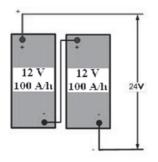
Fig. 2. A serial connection of batteries (general capacity of 100 a/h, voltage 24 V) [2]
